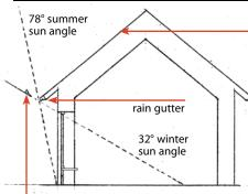
Sun Angles: Pay attention to the construction details when designing your roof overhangs. Rain gutters, window molding, and the distance the window is inset from the outside wall surface will all influence the amount of sunlight that can enter the home. Include these details in your cross-section drawing.
